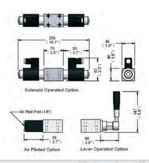
W2 Series ultra low leakage Poppet Directional Valves – CETOP03/DO3/NG6 manifold interface.
