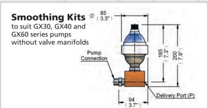
**HEYPAC** pumps are double acting single piston pumps and, as a result, produce small pressure pulsations. These can be significantly reduced by the addition of the appropriate smoothing kit to the outlet port of the pump. For maximum pulsation dampening the accumulator should be installed as close to the outlet port as possible
