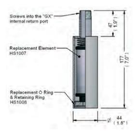
A return line filter, especially suitable for use with manifold equipped GX20, GX30 and GX40 series pumps. The filter screws into the return port (G1/2"BSPT) on the bottom face of the pump flange. It is only suitable for use with R1, R2 and 10 litre capacity reservoirs
