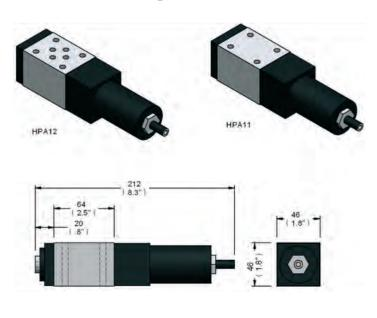
A direct operated CETOP03/DO3/NG6 pressure reducing valve for use with **HEYPAC** pumps. The valve is supplied in either "flange" form (HPA11) for use as a single sub-plate mounted valve or "sandwich" form (HPA12) for use as part of a valve stack. The reduced pressure is adjustable by means of a socket head screw.
