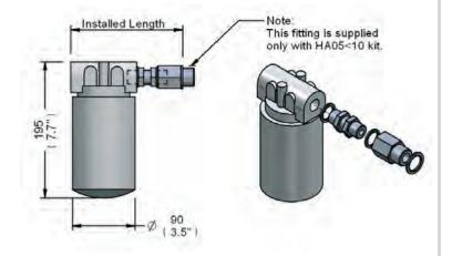
A range of line mounted 10 micron return filters to suit GX05 to GX80 series pumps. The filter is available as a stand-alone item or in a kit, which also contains all necessary fittings to mount the filter to the pump return port.
