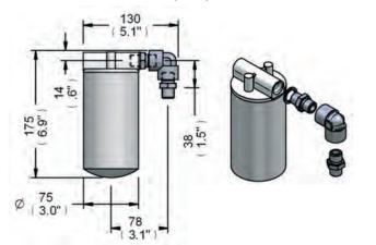
A range of line mounted 10 micron return filters to suit KR05 to KR80 series pumps. The filter is available as a stand-alone item or in a kit, which also contains all necessary fittings to mount the filter to the pump return port.
