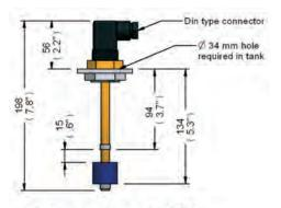
Note: Dimensions shown are for the T10 Stem length for T30 is 50mm longer
