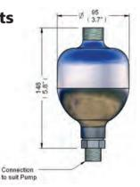
**HEYPAC** pumps are double acting single piston pumps and, as a result, produce small pressure pulsations. These can be significantly reduced by the addition of the appropriate smoothing kit to the outlet port of the pump. For maximum pulsation dampening the accumulator should be installed as close to the outlet port as possible
